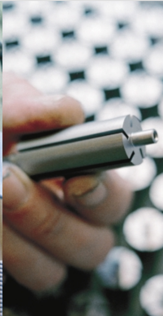
K.M.C. Ytbehandling AB, which is a part of Addtech Production Systems, delivers systems such as surface treatment facilities custom designed to meet customer requirements. The picture shows burr removal with glass beads as the blasting medium.
