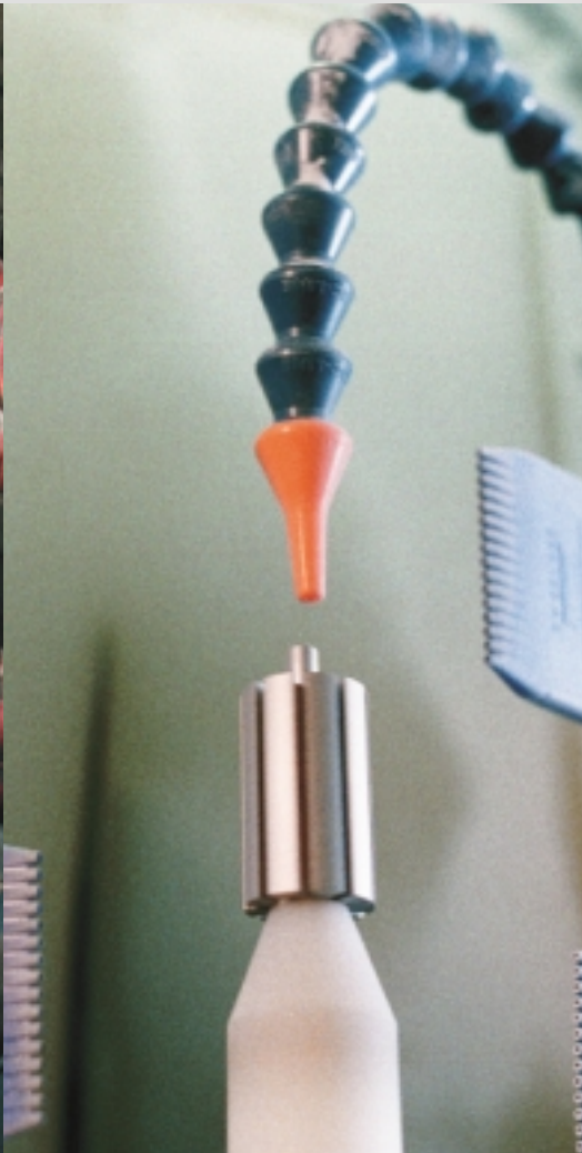
K.M.C. Ytbehandling AB, which is a part of Addtech Production Systems, delivers systems such as surface treatment facilities custom designed to meet customer requirements. The picture shows burr removal with glass beads as the blasting medium.
